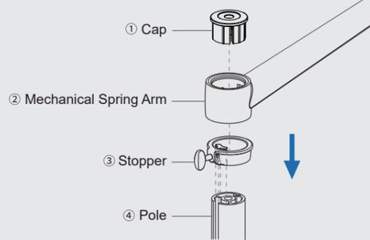
Note: Install the mechanical arm and the stopper on the pole as shown.
