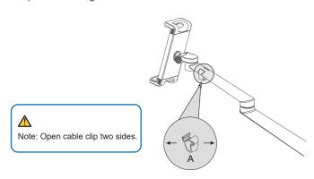
Slide the plastic cover on the lower link upwards until it diengages, then remove (A). Put power and monitor cables into the plastic cover (B). Then slide the cover downwards until click into place (C).
