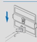
Insert the Laptop Plate into the groove, when heard a click sound means done.
