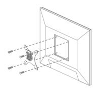
1 As the picture shows, install VESA mount on monitor. Be careful to leave the slide clip upwards.
