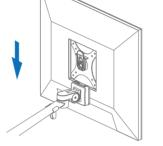
2 Insert the VESA connector into the groove, when heard a click sound means done.
