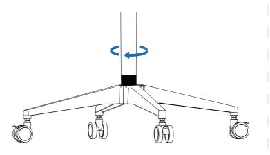
If you feel the feet not stable or need to elevate the feet height, you can adjust the screw nut as picture. 1 Lower nut: Loose it to adjust the height.
