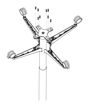
To install four aluminum feet with wheels, tighten the screws to fasten it with the vertical prop.
