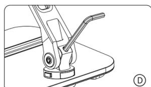
Using the medium wrench, adjust the tightness of the support bar.
